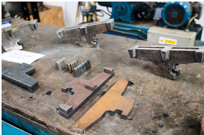
Fabrication of the grate bars under way.
