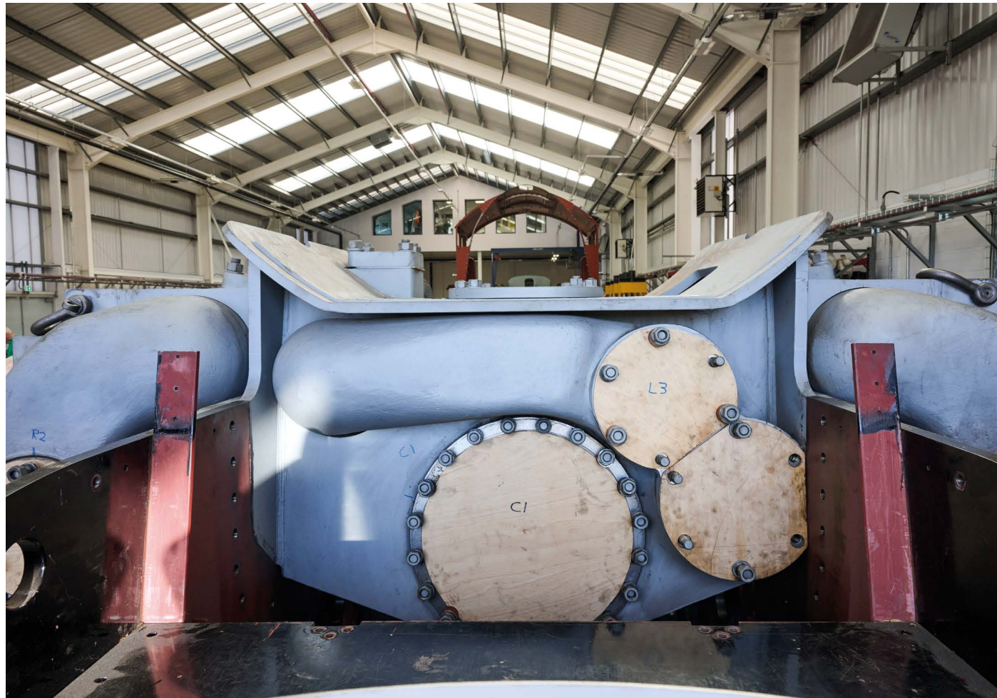
The monobloc sits comfortably between the P2's frames.
