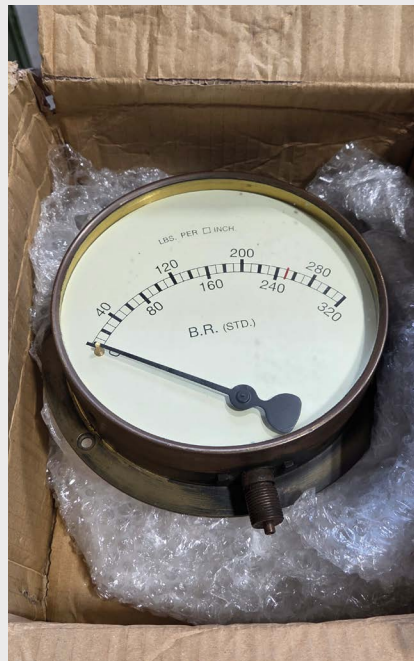
One of a pair of 320psi pressure gauges acquired for No. 2007.
