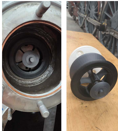
One of the printed 'double beat' valves is offered up to the block.
